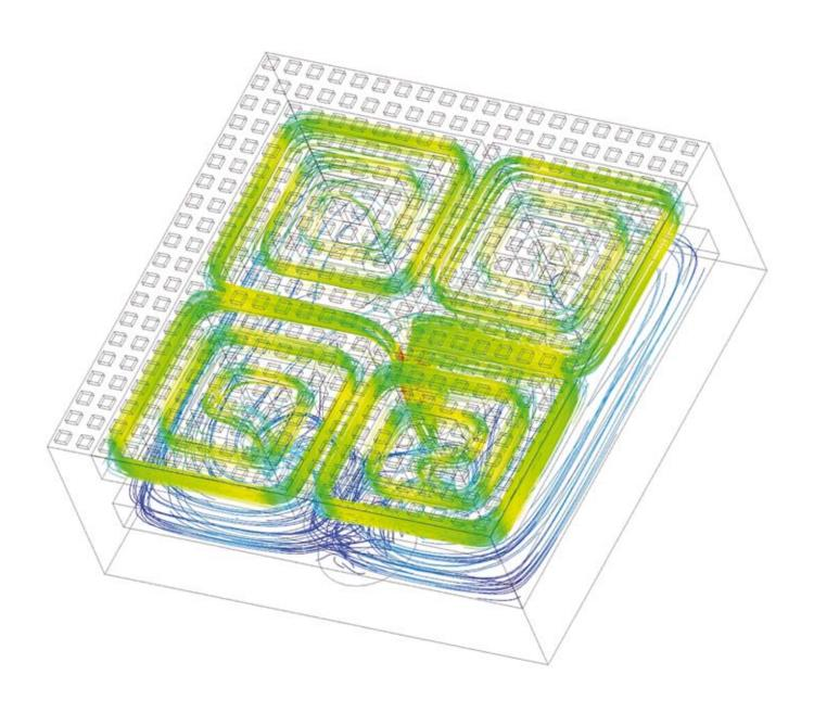
Velocity distribution of cooling liquid within ceramic
